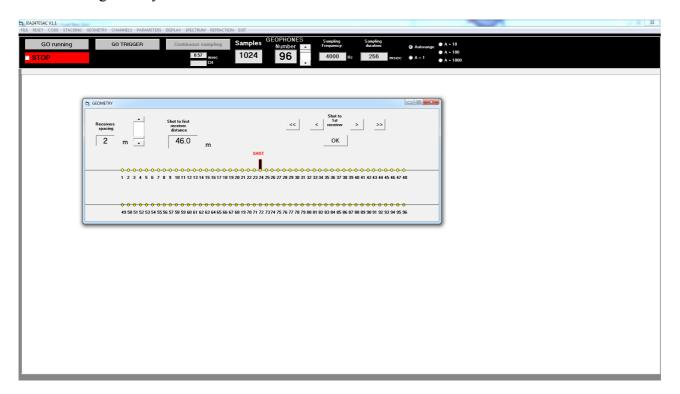
Set the distance between geophones (which in the example is four meters) and the position of the trigger with respect to the first unit (now 46 meters to the right of first unit).
