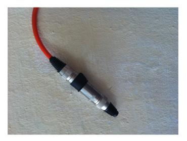
Termination simply consists of a resistor of 120ohm, necessary for correct line termination of cable. If you do not terminate the line in this way, signal reflections make impossible any transmition,
