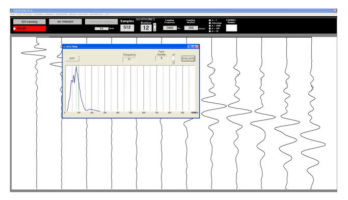
Being 2000Hz the acquisition frequency, the maximum frequency of 1000Hz is displayed in the graph, in accordance with the sampling theorem.
