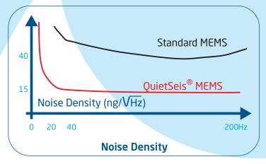
On the mechanical side, meanwhile, the MEMS vacuum was increased further to lower the Brownian noise. Moreover, a detailed analysis of all spurious high-frequency modes was performed. Mechanical design was modified to mitigate all aspects that could impact system noise performances.
