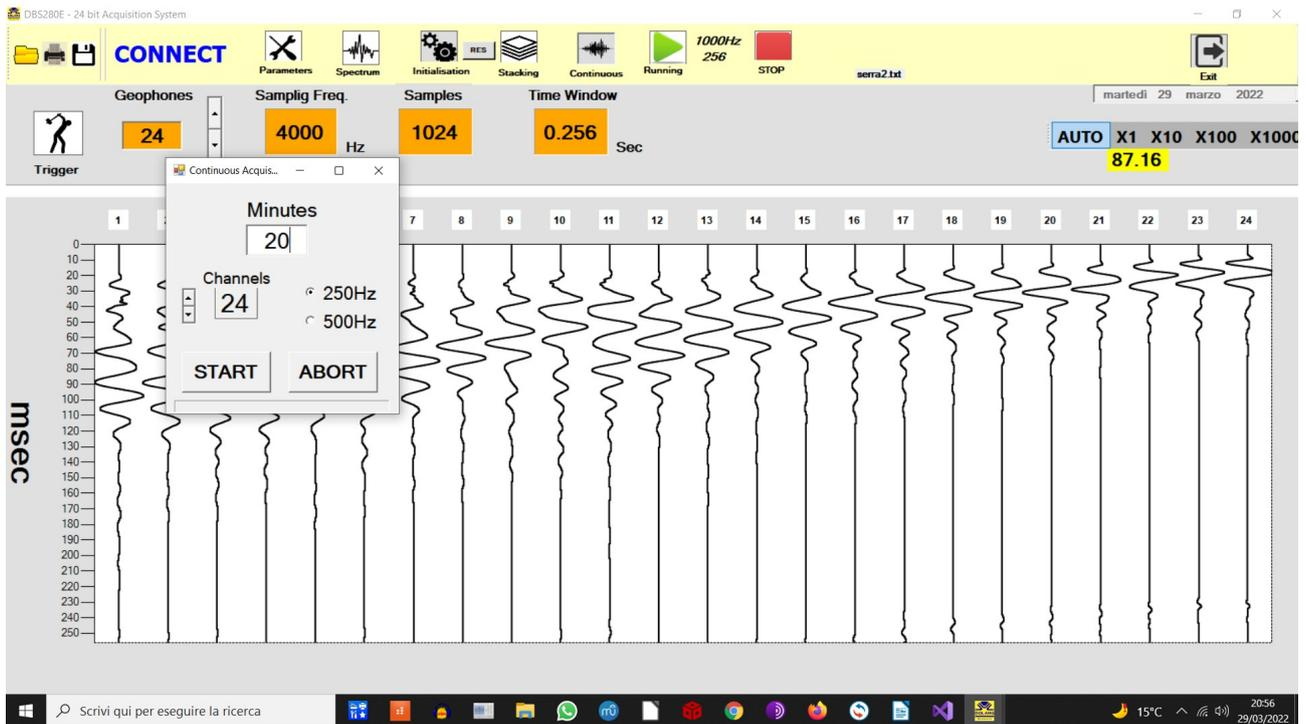
At the end of acquisition, file can be saved as sg2 and sgy format.
