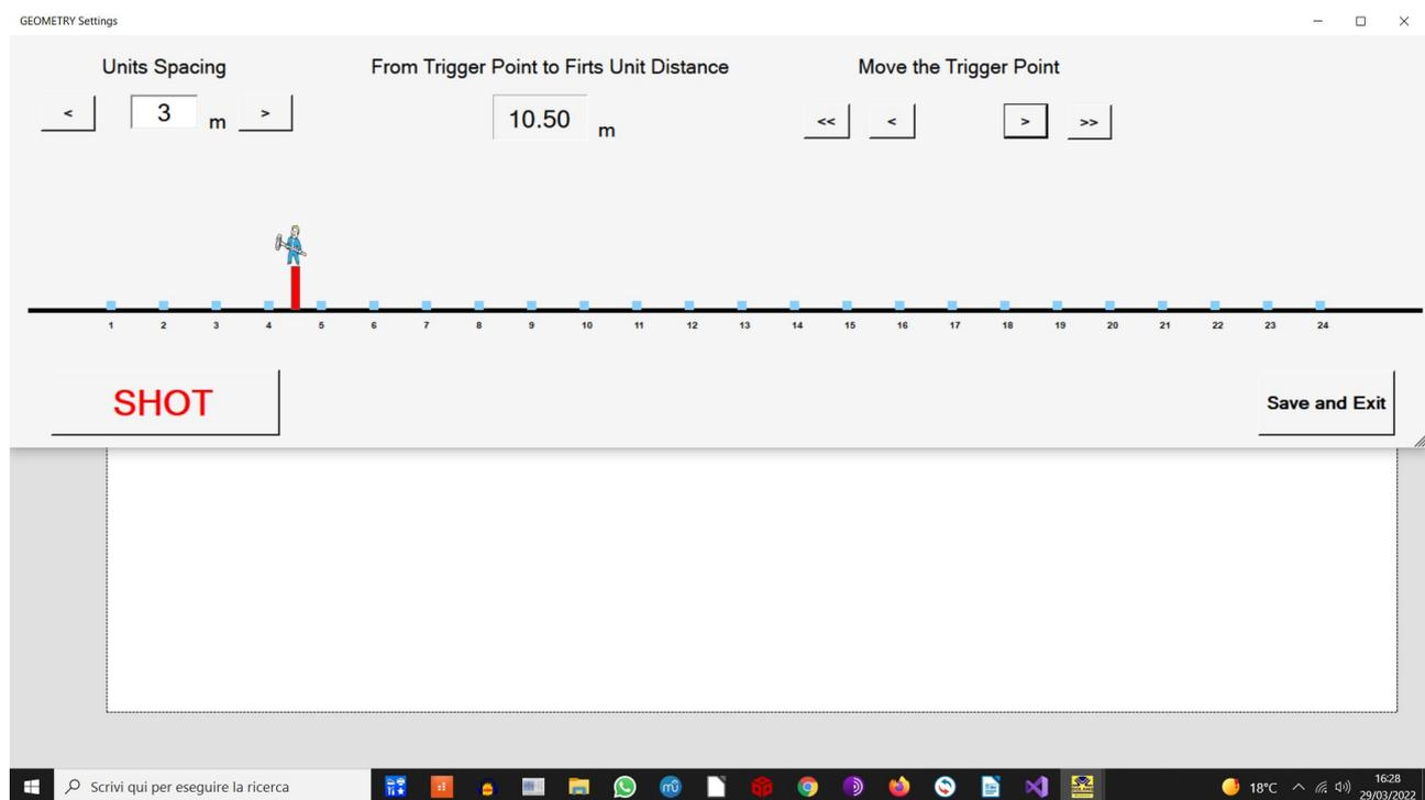
Set the distance between geophones (which in the example is 3 meters) and the position of the trigger point, respect to the first unit.
