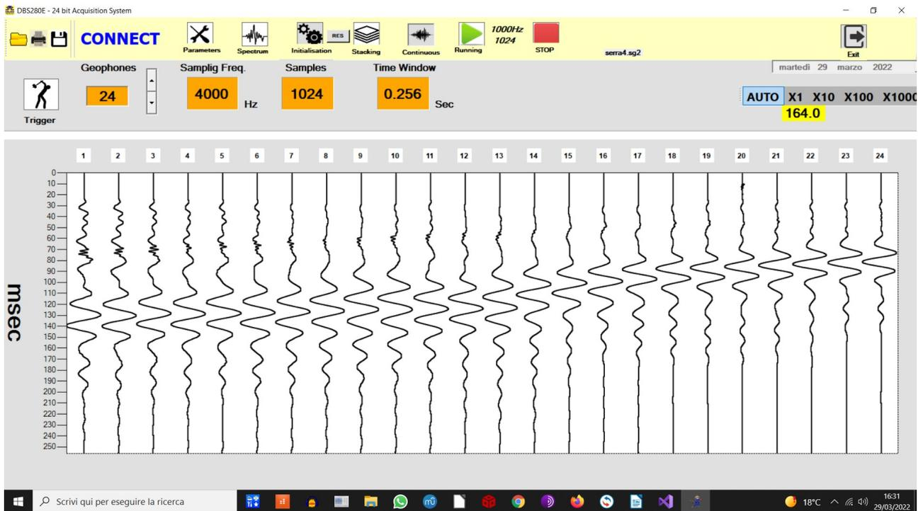
Moving the mouse over a point in a track, in a top right yellow window will be visible the relative time from trigger instant.
