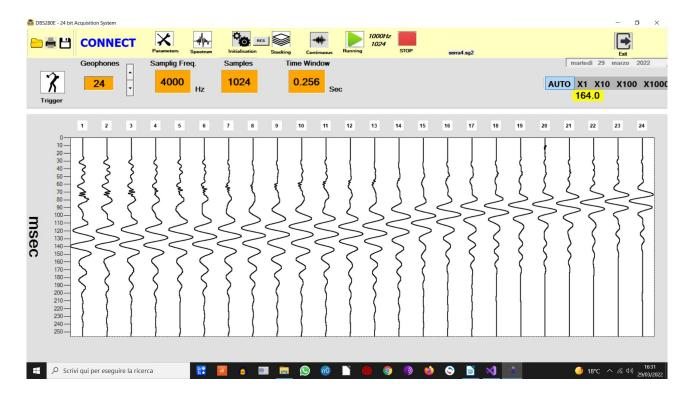
Moving the mouse over a point in a track, in a top right yellow window will be visible the relative time from trigger instant.
