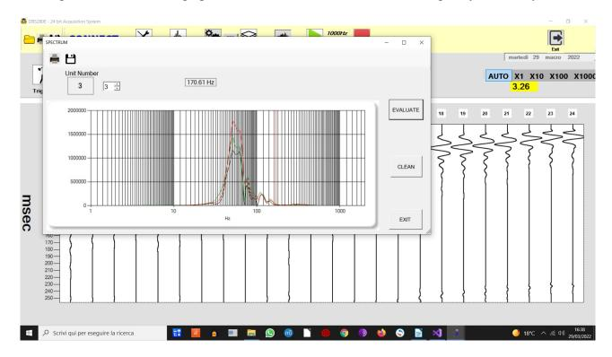
Being 4000Hz the acquisition frequency, the maximum frequency of 1500Hz is displayed in the graph, in accordance with the sampling theorem, that does not allow meaningful frequencies above half sampling frequency value.
