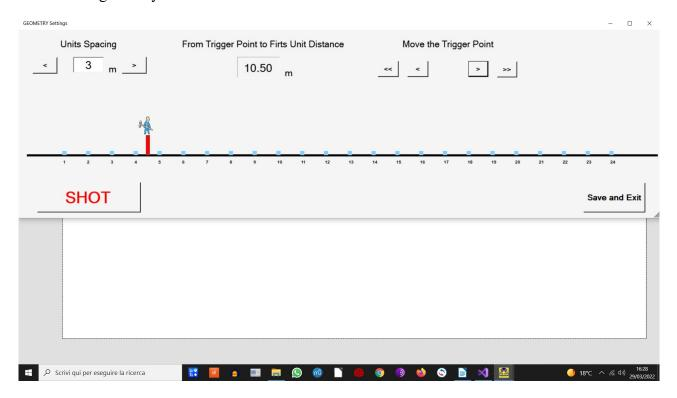
Set the distance between geophones (which in the example is 3 meters) and the position of the trigger point, respect to the first unit.
