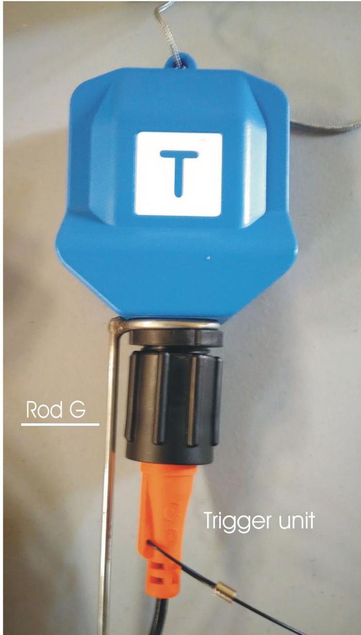
*Trigger Unit with wire connected*
