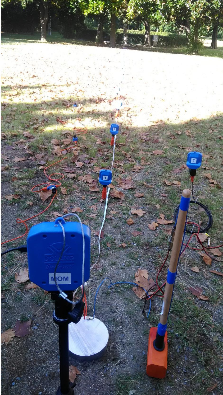
*TRG plate is positioned with some offset from Unit 1; TGR unit is aside. waiting for the triaer.*
